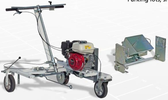
Hand-guided self-propelled road marking machine developed for processing 2-component cold plastics either in form of structural or flat marking. Absence of automatic glass beads system makes 2KPPM the best choice for parking lots marking. This machine lets you stripe in 3,5 cm distance from curb.
