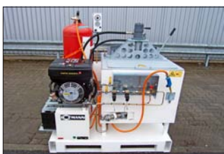
② ID100 - Compact, transportable unit consisting of preheater and power station
